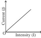
The intensity of incident light affects the photoelectric current but leaves the maximum kinetic energy of photoelectrons unchanged.
